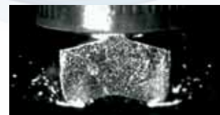
Image of a High Speed Current projection weld
