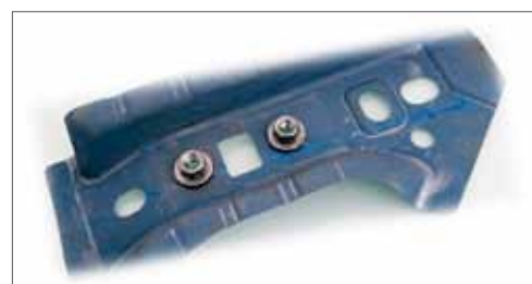
Example of a HSC projection weld
