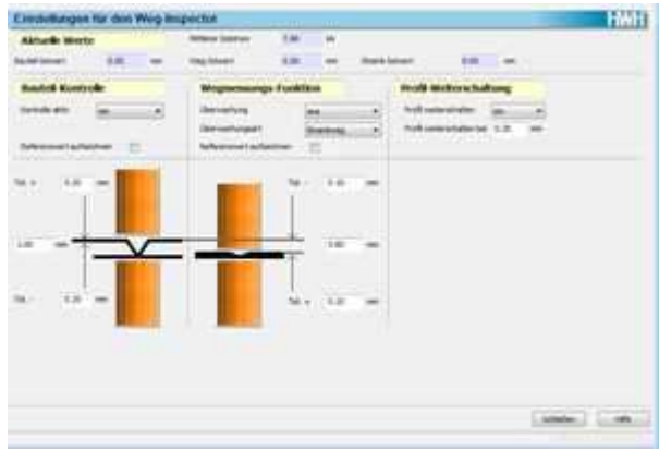
Fig. 2-4 Settings for the distance inspector via the XPegasus user interface
