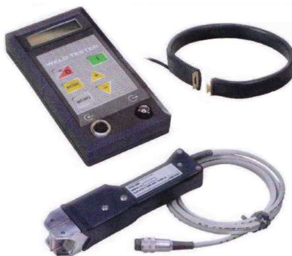
Fig. 13-2 TE1600 with Rogowski belt and force measuring probe
