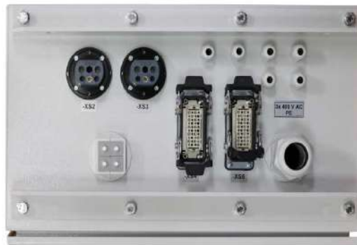
Fig. 5-6 Wall-mounted spot welding system, connections
